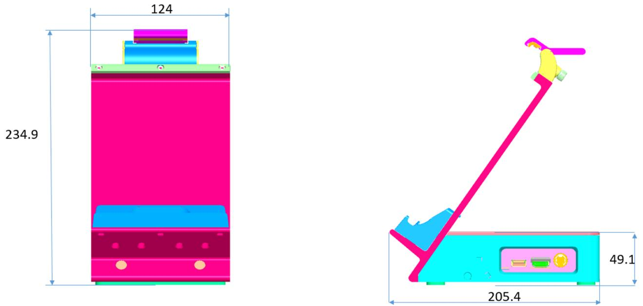
**Figure2: MiTAC Cappuccino Docking Station Dimension (without Cable Cover)**
